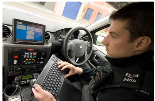
The ROADSTER-M1 is designed especially for use in a moving vehicle coping well with varying voltages and temperatures. The unit supports both 12V and 24V vehicles and there is an on-board controlled start-up and Windows shut-down procedure.
