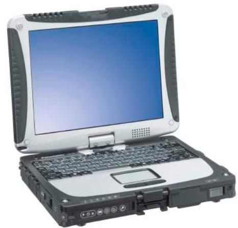
Battery or mains powered, the PC has an Intel i5 processor and can connect to two RoadWolf HD or RoadWolf Nano HD ANPR Cameras which can be mounted on a vehicle roof bar or a tripod.
