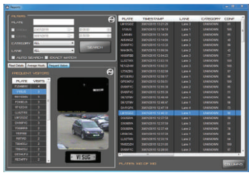
RPX-LIVE: Search by a full or partial plate, lane, date, time or database category
